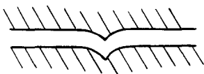
Figure 12 Schematic drawing of profile of crack arrest line in epoxy specimens showing deviation of crack line from main fracture plane (after Phillips et al. [16]).
